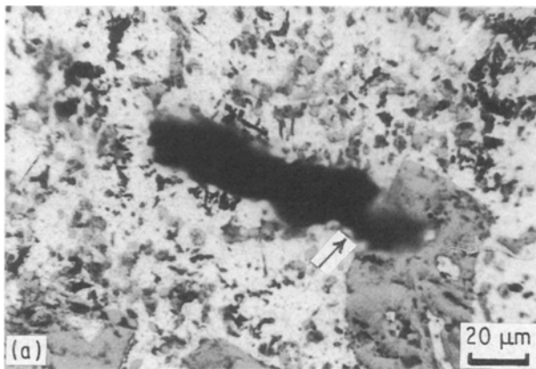
Figure 3 Microstructures of the composite after ageing at 180°C for (a, b) 8 h and (c) 16 h. Increased extent of spheroidization of the eutectic silicon and the complex intermetallic phases (a) and fragmentation of primary silicon particles (arrowed in b) may be noted. A typical example of the entanglement of the primary silicon with graphite is evident in (a) (arrowed) while coarsening of the phases may be seen in (c).
