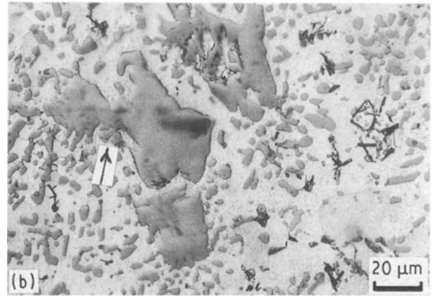
Figure 2 Micrographs of the composite after solution treatment at 516°C for 7 h revealing (a) the breaking of the as-cast dendritic structure of the matrix and spheroidization of the eutectic silicon particles, and (b) the modification in the morphology of the complex intermetallic compound over the as-cast state and refinement of the primary silicon phase through fragmentation (arrowed).
